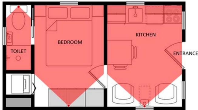
Figure 44. The first configuration of the home sensors network of Case Study 2.
