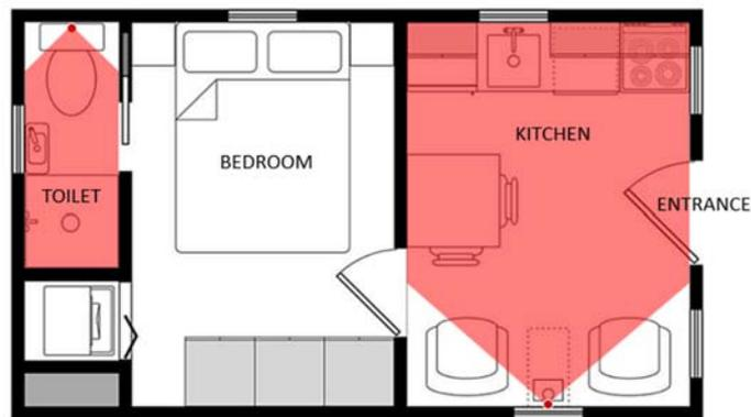
Figure 45. The second configuration of the home sensors network of Case Study 2.
