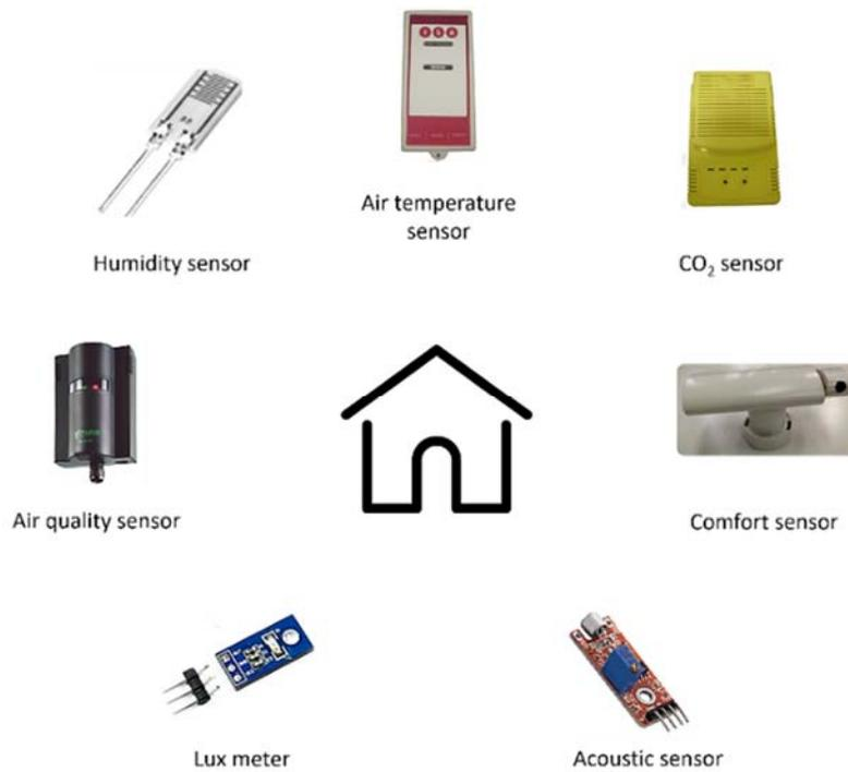
Figure 19. Sensor network for IEQ monitoring in the living environment.
