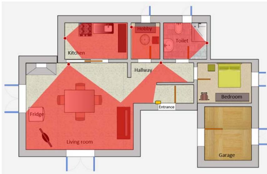
Figure 43. The third configuration of the home sensor network of Case Study 1.
